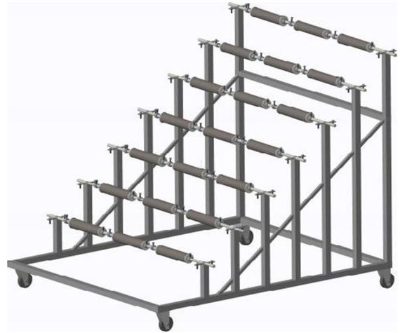
FIG.3 THREE-DIMENSIONAL VIEW OF WARP CREEL
