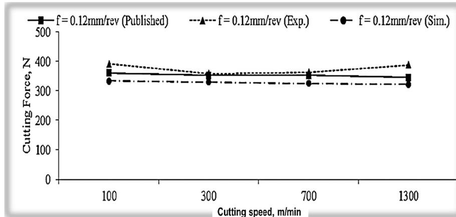
FIGURE 12. COMPARISON OF EXPERIMENTAL AND SIMULATED CUTTING FORCE, FC WITH THE PUBLISHED RESULTS AT THE FEED RATE,  $F = 0.12\text{MM/REV}$
