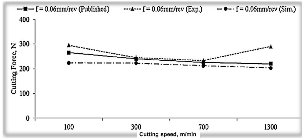
FIGURE 10. COMPARISON OF EXPERIMENTAL AND SIMULATED CUTTING FORCE,  $F_c$  WITH THE PUBLISHED RESULTS AT THE FEED RATE,  $F = 0.06\text{MM/REV}$
