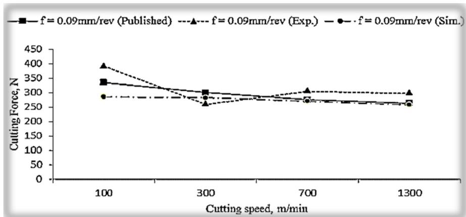
FIGURE 11. COMPARISON OF EXPERIMENTAL AND SIMULATED CUTTING FORCE,  $F_c$  WITH THE PUBLISHED RESULTS AT THE FEED RATE,  $F = 0.09\text{MM/REV}$
