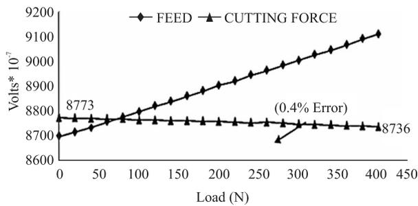
FIG. 5. FEED FORCE ARM CALIBRATION
