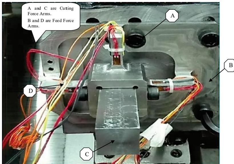
FIG. 3. FABRICATED DYNAMOMETER WITH INSTALLED STRAIN GAUGES
