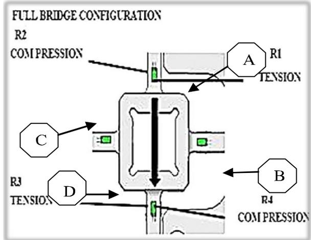
FIG 7(B).TOP VIEW OF FULL BRIDGE CONFIGURATION
