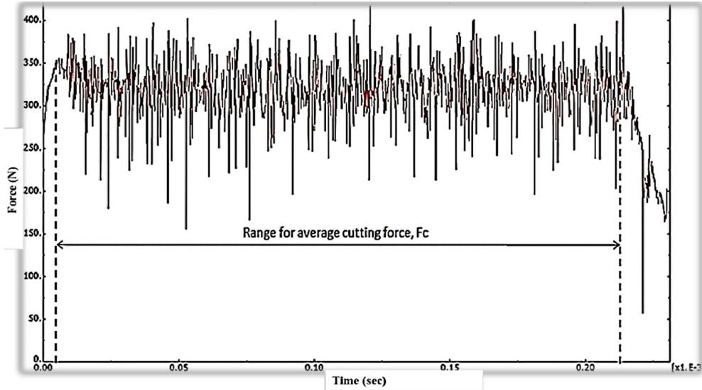
FIG. 9. CUTTING FORCE,  $F_c$  AT  $V = 1300\text{M/MIN}$  AND  $F = 0.12\text{MM/REV}$
