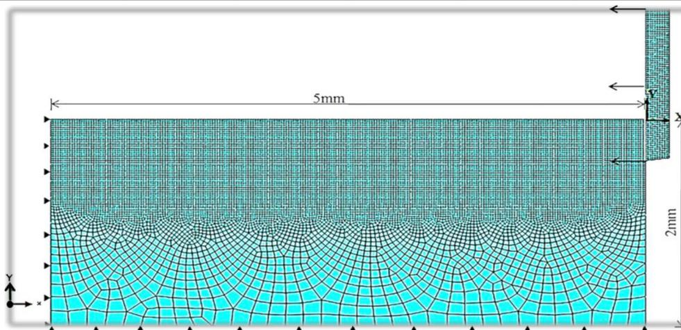
FIG. 8. FINITE ELEMENT MESHING AND BOUNDARY CONDITIONS SHOWING FIXED WORKPIECE AND TOOL VELOCITY GIVEN ALONG X-AXIS [6].
