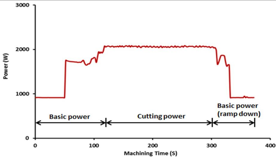
FIG. 4. POWER PROFILE MILLING EXPERIMENT
