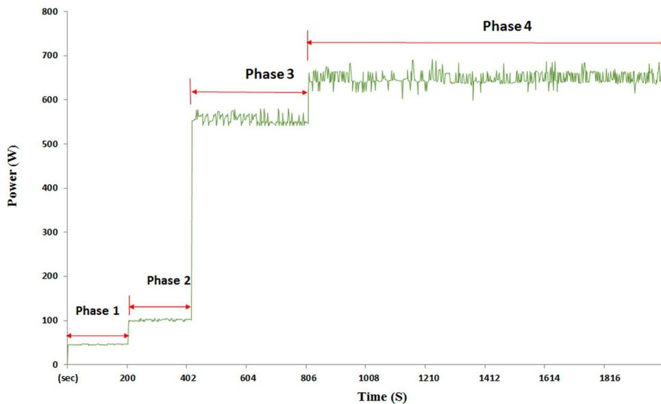
FIG. 2. POWER PROFILE TOPSCNC WIRE-CUT EDM MACHINE
