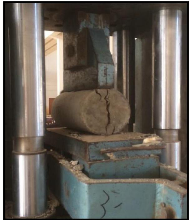
*FIG. 7. COMPRESSIVE STRENGTH TEST SETUP*
