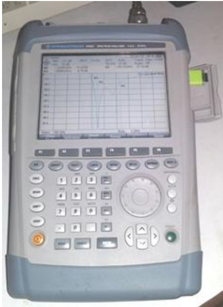
FIG. 9. VECTOR NETWORK ANALYZER USED FOR TESTING PURPOSES
