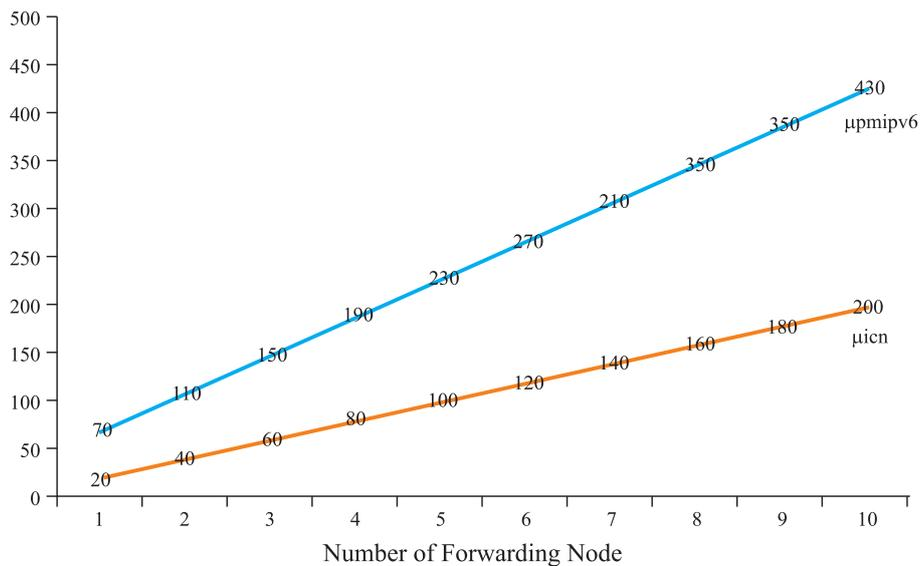
FIG. 4. SERVICE RECOVERY TIME FOR ICN AND PMIPv6 VERSUS NUMBER OF FORWARDING NODE
