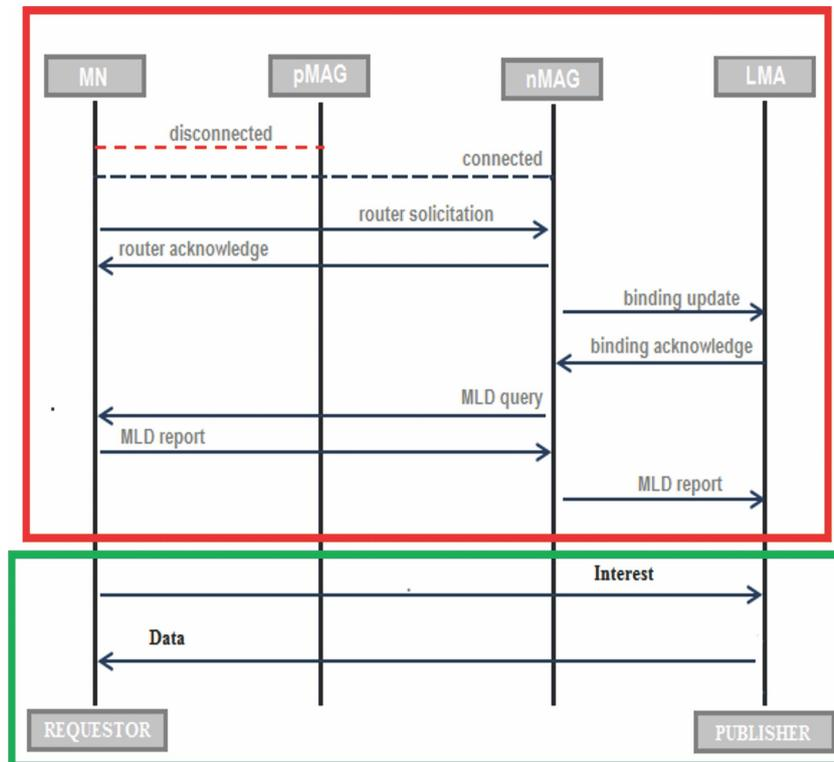
FIG. 2. MN HANDOVER SIGNALING FLOW
