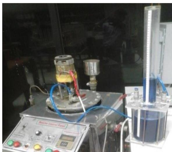
FIG. 2. CSTR WITH METHANE MEASURING JAR
