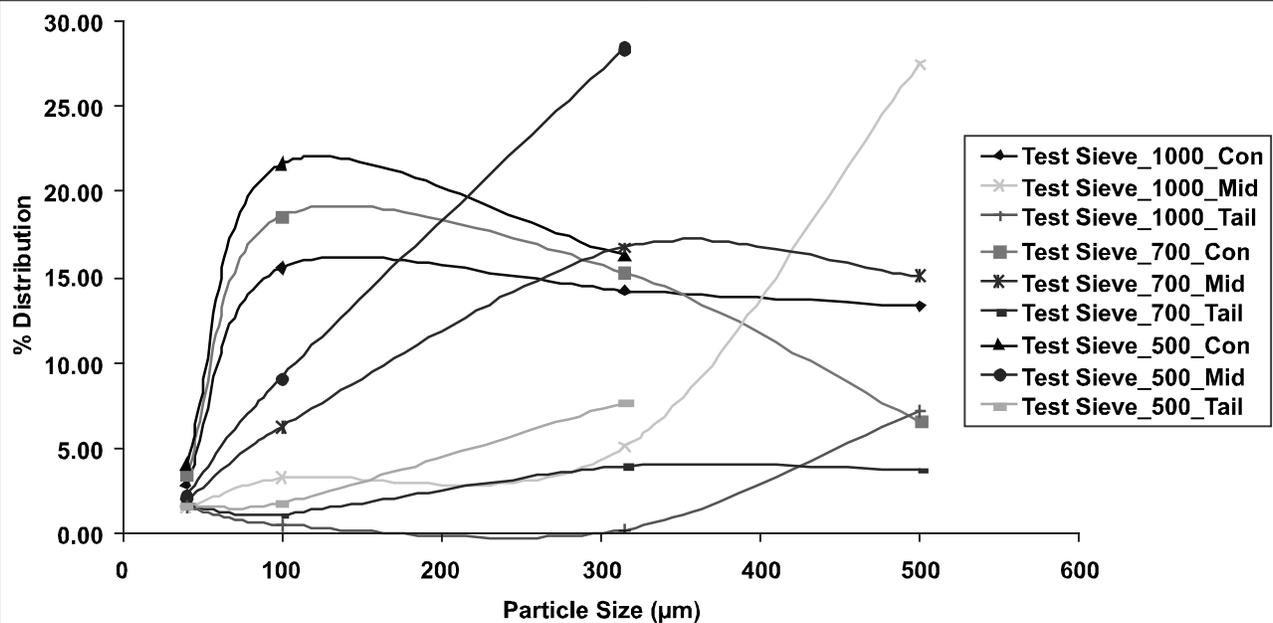
FIG. 5. PERCENT DISTRIBUTION OF PARTICLES IN CONCENTRATE, MIDDINGS, AND TAILINGS AT DIFFERENT FEED SIZES
