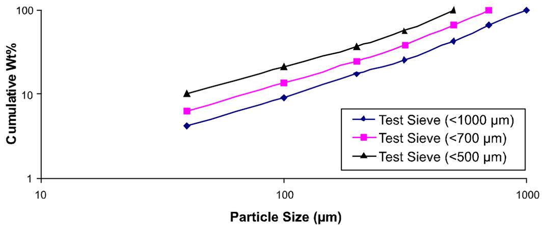
FIG. 4. PARTICLE SIZE DISTRIBUTION OF PRODUCT MATERIAL AT TEST SIEVE 1000, 700 AND 500μm
