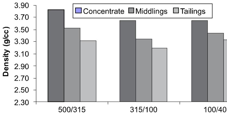
FIG. 8. DENSITY OF DIFFERENT PARTICLE SIZE FRACTIONS OBTAINED AT 500 $\mu$ m TEST SIEVE
