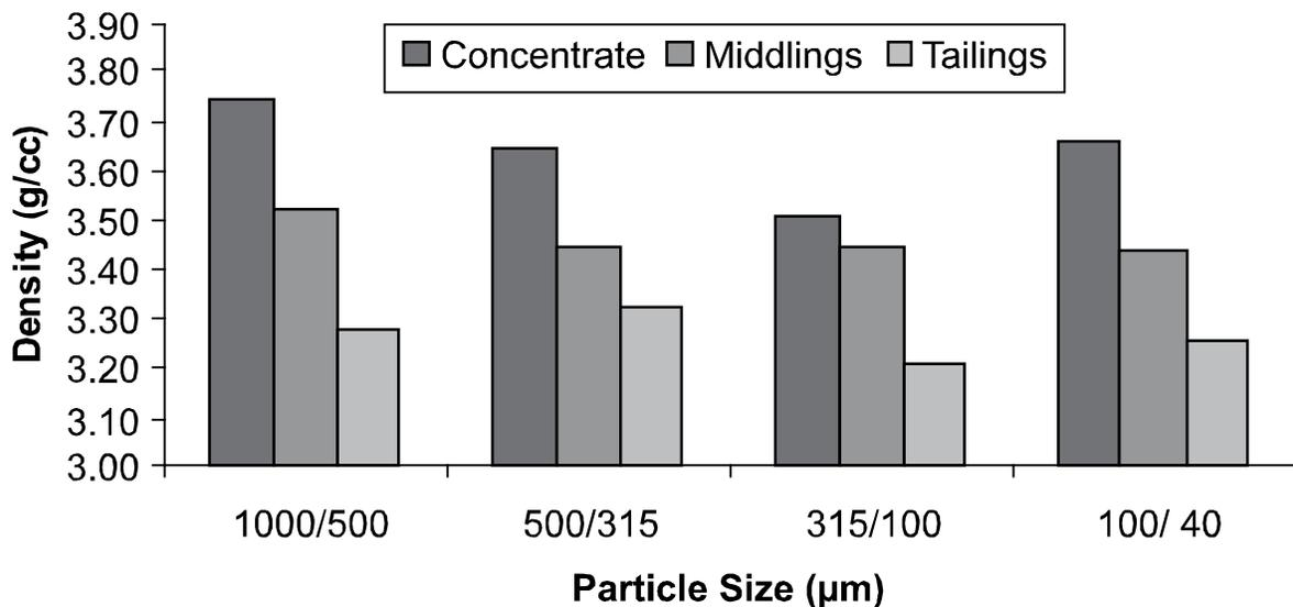
FIG. 6. DENSITY OF DIFFERENT PARTICLE SIZE FRACTIONS OBTAINED AT 1000 $\mu\text{m}$  TEST SIEVE
