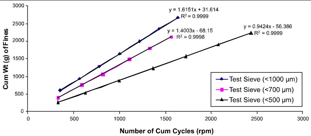
FIG. 2. WT% OF SPECIFIC FINES PRODUCED DURING ROD MILL GRINDING AT 1000, 700 AND 500μm TEST SIEVES
