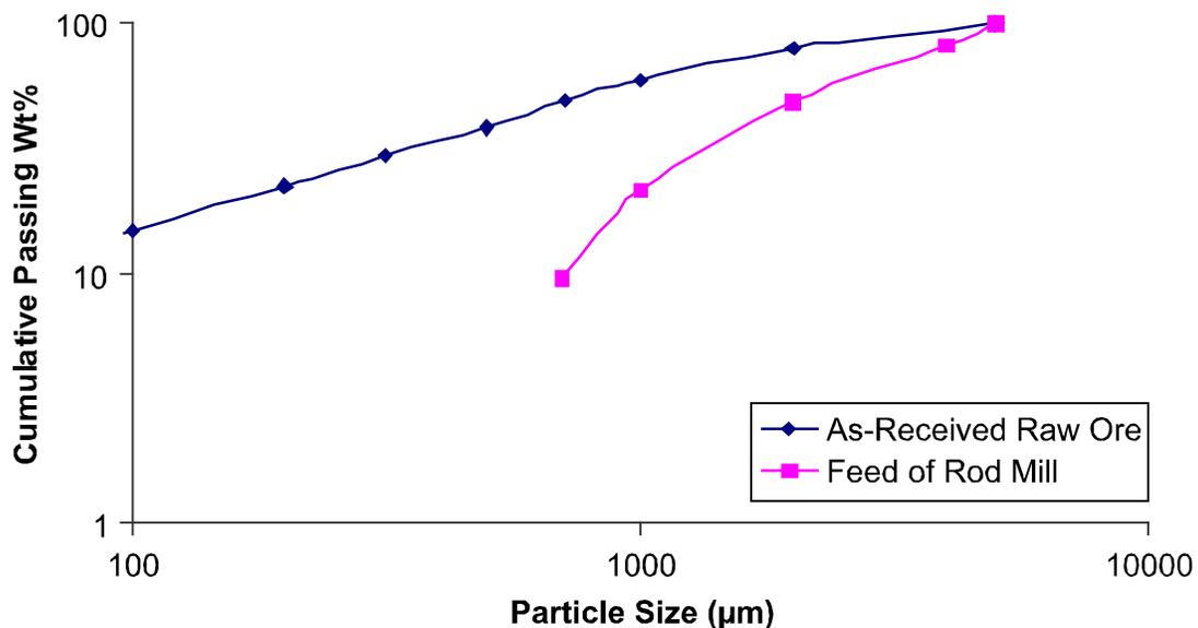
FIG. 1. PARTICLE SIZE DISTRIBUTION OF AS RECEIVED RAW AND FEED ORE USED FOR ROD MILL GRINDING
