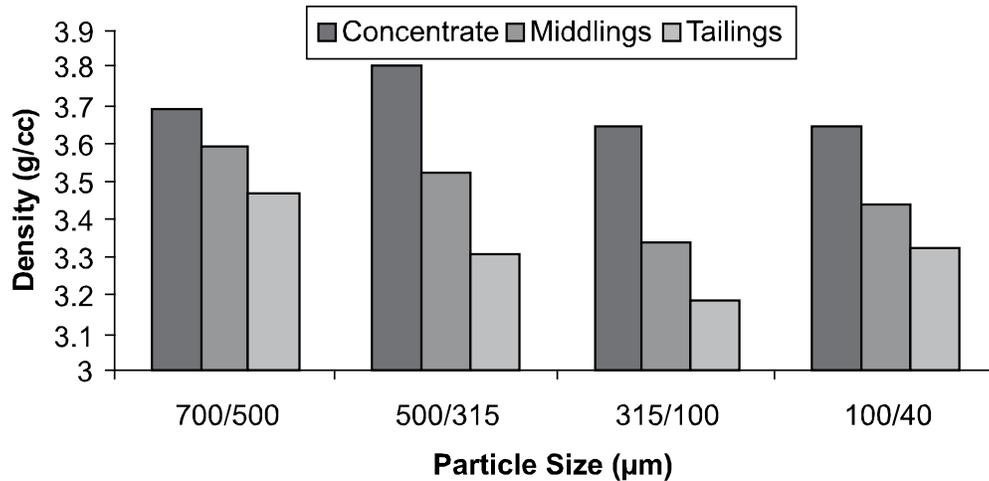
FIG. 7. DENSITY OF DIFFERENT PARTICLE SIZE FRACTIONS OBTAINED AT 700 $\mu$ m TEST SIEVE
