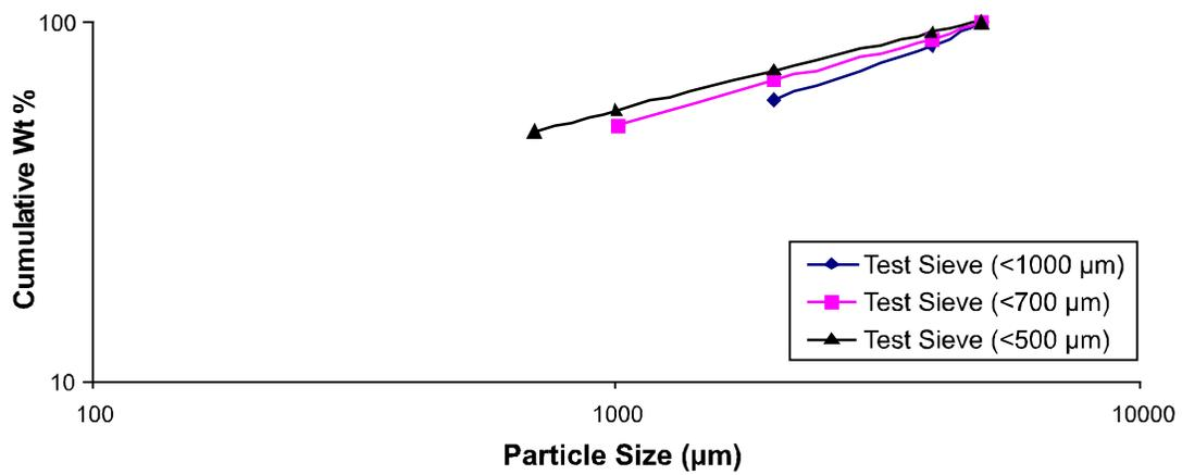
FIG. 3. PARTICLE SIZE DISTRIBUTION OF FEED/RECYCLED MATERIAL AT TEST SIEVE 1000, 700 AND 500μm
