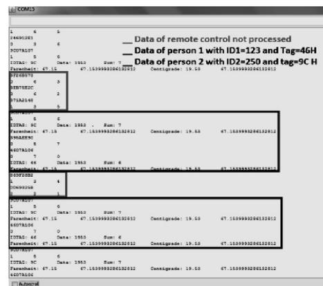
FIG. 4. RECIEVER'S RESPONSE IN PRESENCE OF INTERFERENCE SIGNALS WHEN ID1 OR ID2 AND REMOTE CONTROL TRANSMITTING THE DATA
