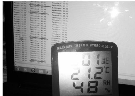
FIG. 1(a). TEMPERATURE READING VERIFICATION WITH THE HELP OF DIGITAL HYGRO THERMOMETER
