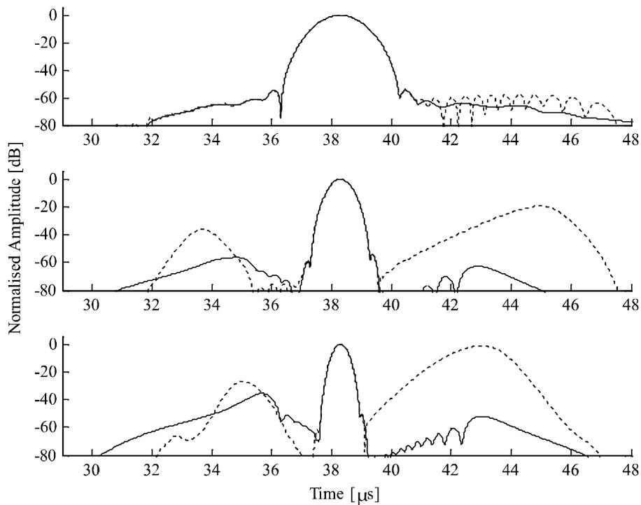
FIG. 8. THE COMPARISON OF UNFILTERED (DASHED LINE) AND FRFT PRE-FILTERED (SOLID LINE) HARMONIC MATCHED FILTERED COMPRESSED SIGNALS OBTAINED USING CHIRP EXCITATION WITH  $-6\text{dB}$  FRACTIONAL BANDWIDTH OF 22.6% (TOP), 44.2% (MIDDLE) AND 66.7% (BOTTOM) RESPECTIVELY
