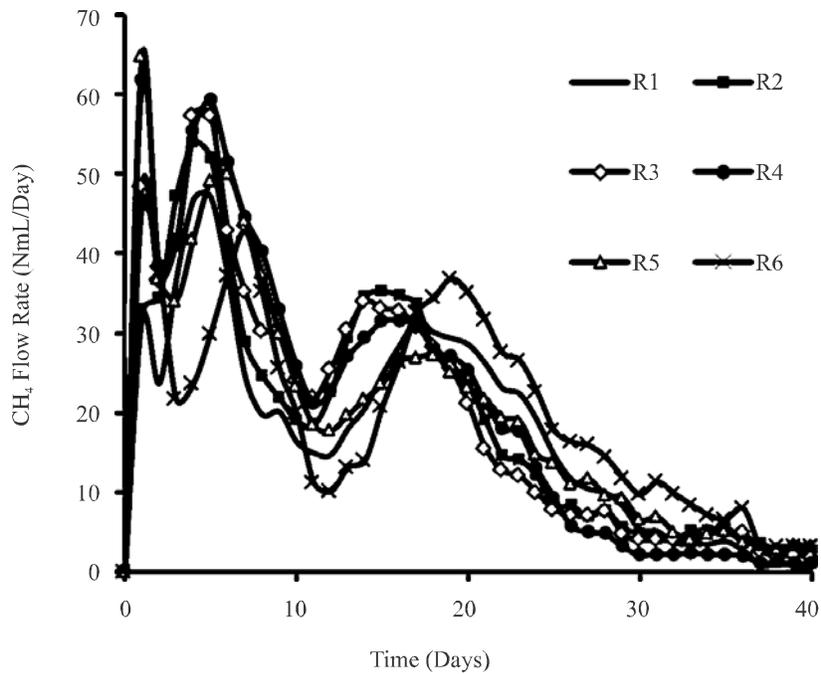
(b) METHANE FLOW RATE; (R1= 10:90; R2= 20:80; R3= 30:70; R4= 40:60; R5= 50:50; R6= 60:40)
