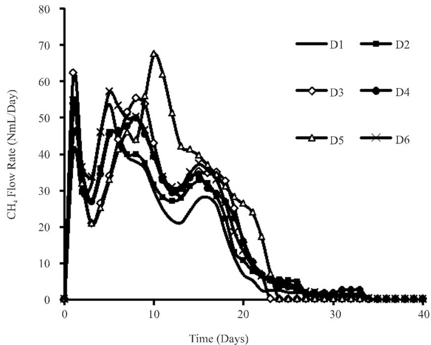
(b) METHANE FLOW RATE; (D1=0.2; D2=0.3; D3=0.4; D4=0.5; D5=0.6; D6=0.7 gNaHCO<sub>3</sub>/gVS)
