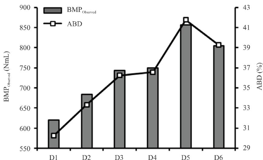
FIG. 5. COMPARISON OF BMP AND ABD AT DIFFERENT ALKALINE DOZES; (D1=0.2; D2=0.3; D3=0.4; D4=0.5; D5=0.6; D6=0.7 gNaHCO<sub>3</sub>/gVS)
