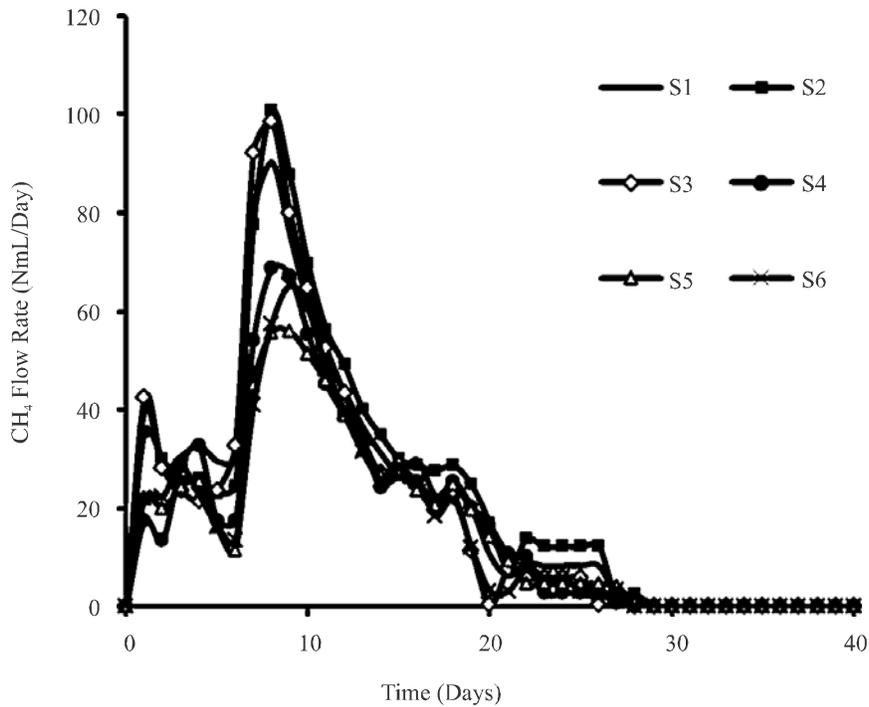
(b) METHANE FLOW RATE; (S1<1; S2=2; S3=4; S4=6; S5=8; S6=10mm)
