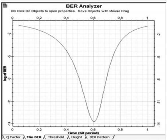
FIG. 5. EDFA MINIMUM BER WITH SMF AND DCF AT 60KM
