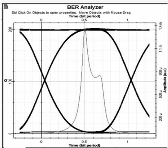
FIG. 4. RAMAN AMPLIFIER'S EYE DIAGRAM AT 60KM
