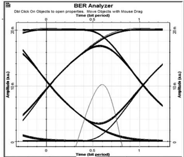
FIG. 3. EDFA EYE DIAGRAM IN CONJUNCTION WITH SMF AND DCF AT 60KM
