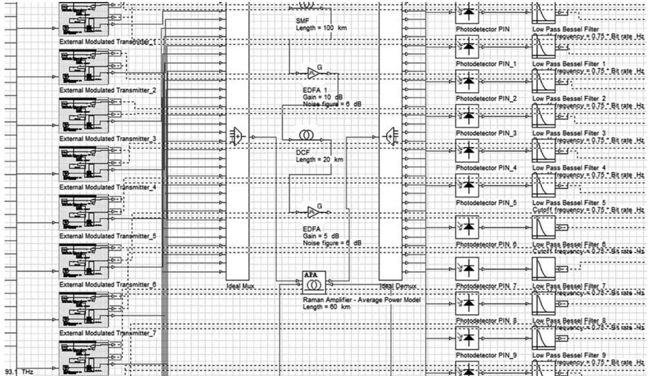
FIG. 2. 32-CHANNEL DWDM SYSTEM DESIGN MODEL USING EDFA AND RAMAN AMPLIFIERS
