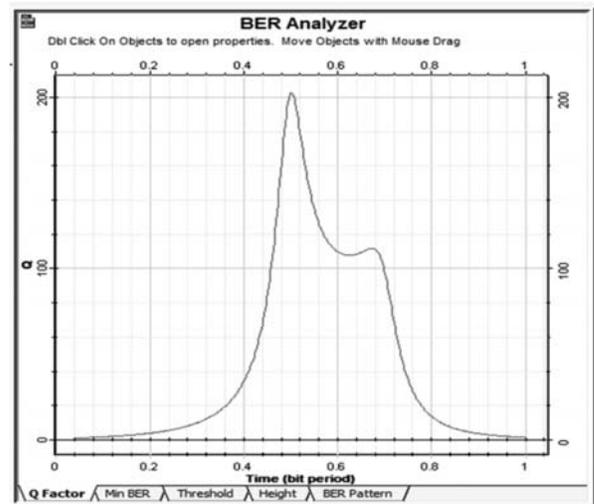
FIG. 8. Q-FACTOR OF RAMAN AMPLIFIER AT 60KM
