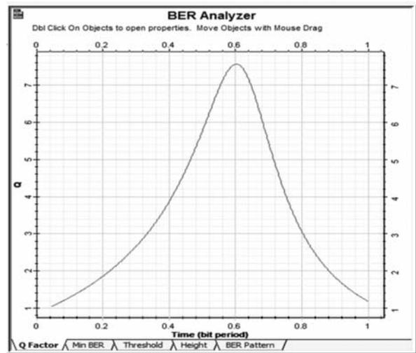
FIG. 7. EDFA Q-FACTOR ALONG WITH SMF AND DCF AT 60KM
