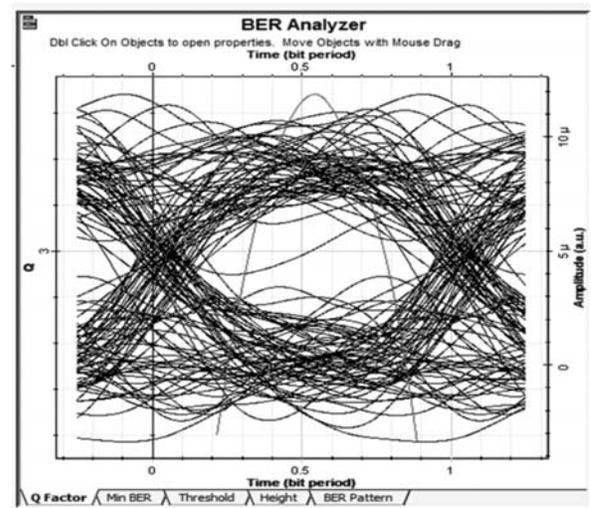
FIG. 14. RAMAN AMPLIFIER PERFORMANCE AT 170KM
