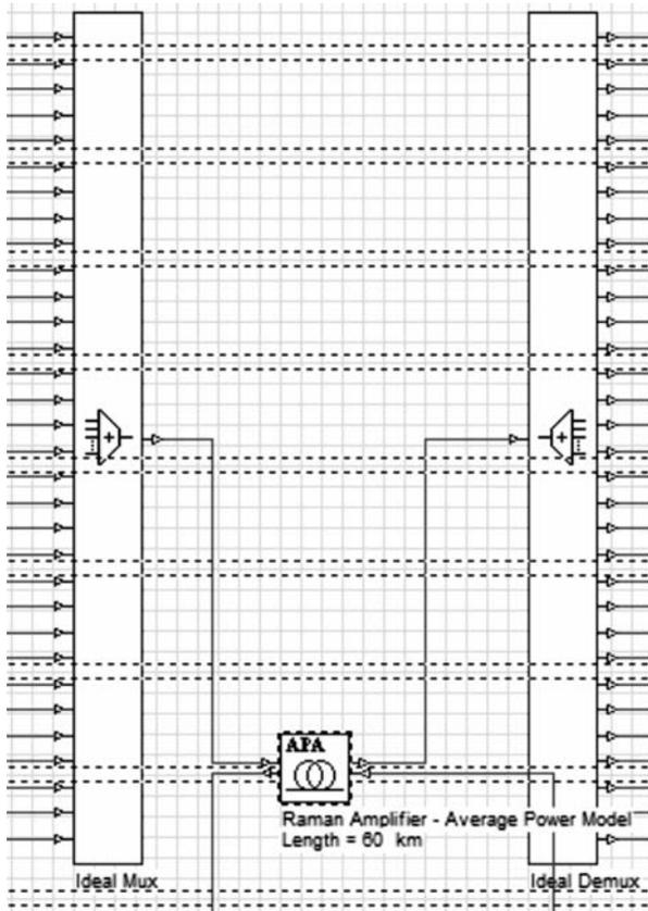
FIG. 1. RAMAN AMPLIFIER MODEL FOR 32-CHANNEL DWDM SYSTEM
