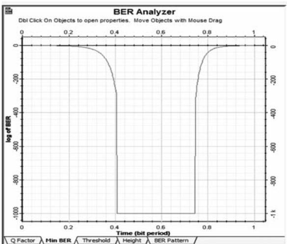
FIG. 6. RAMAN AMPLIFIER'S MINIMUM BER AT 60KM
