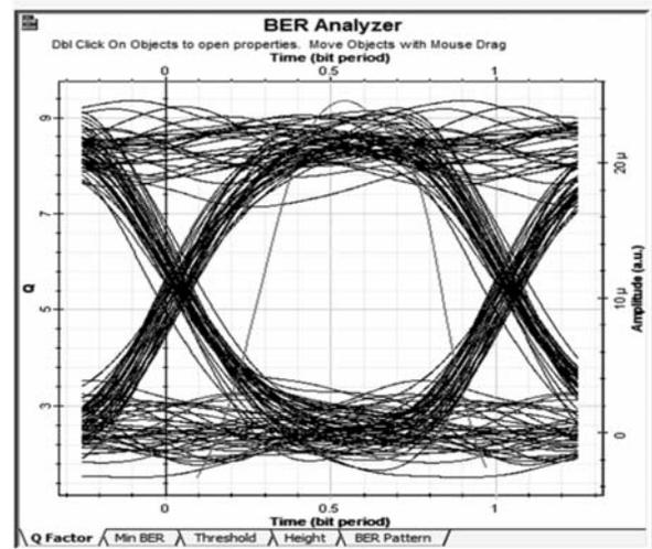
FIG. 13. RAMAN AMPLIFIER PERFORMANCE AT 150KM
