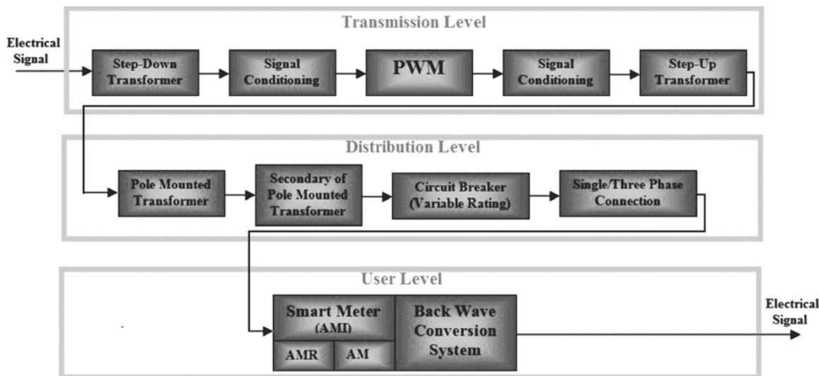
FIG. 1. BLOCK DIAGRAM OF PROPOSED SOLUTION
