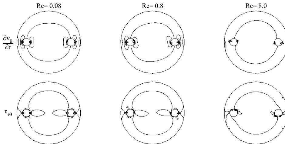
FIG. 2. CONTOURS OF VELOCITY GRADIENTS AND SHEAR STRESSES AT DOUBLE SPEED OF STIRRERS
