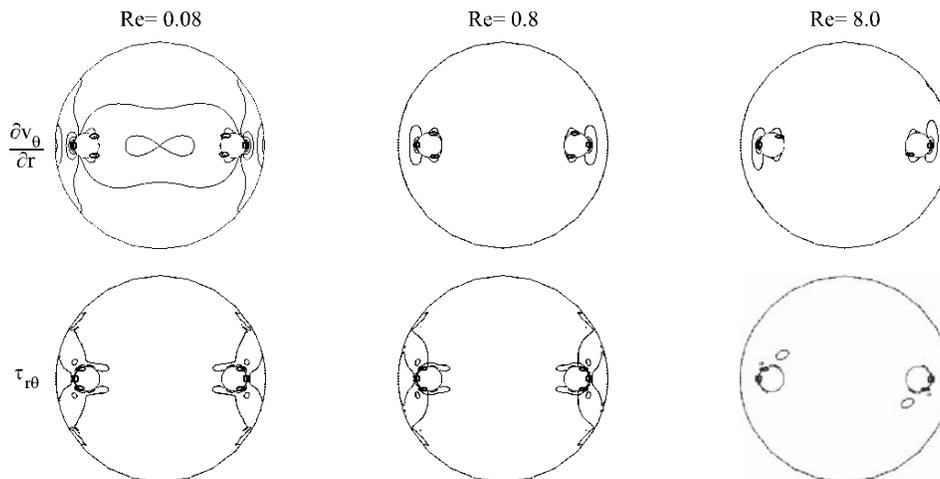
FIG. 1. CONTOURS OF VELOCITY GRADIENTS AND SHEAR STRESSES AT HALF SPEED OF STIRRERS
