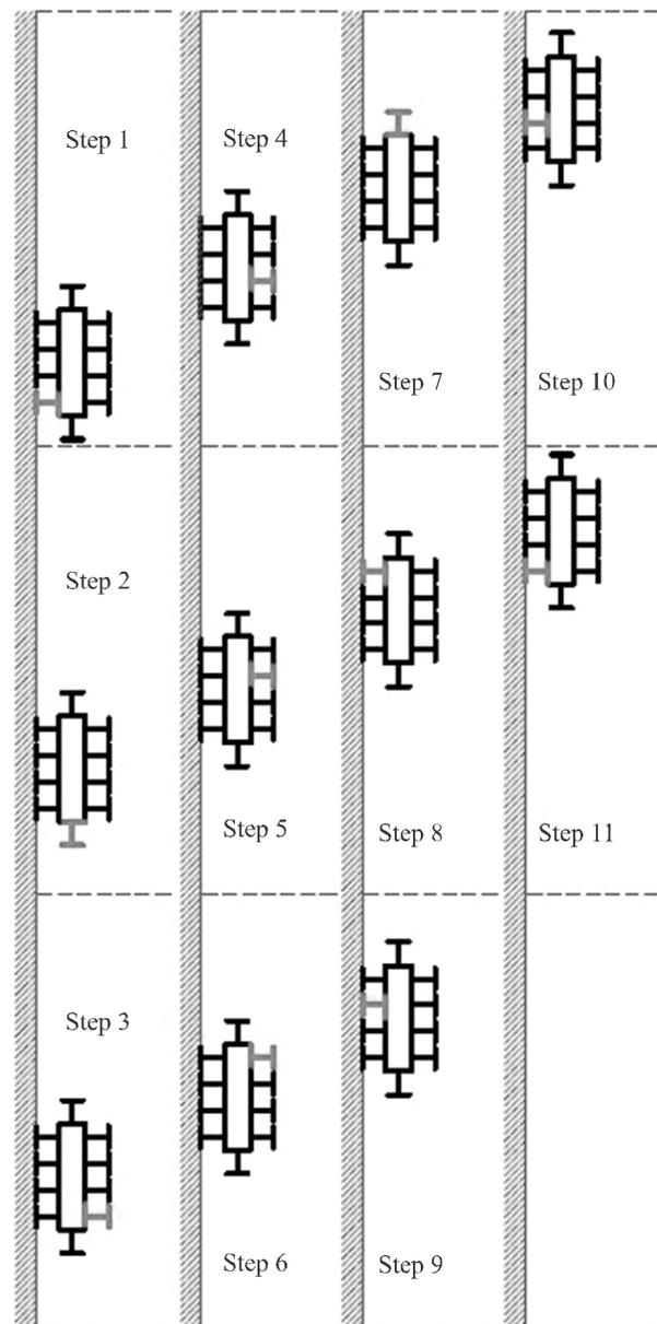
FIG. 8. THE WHEELING GAIT ON VERTICAL TERRAIN
