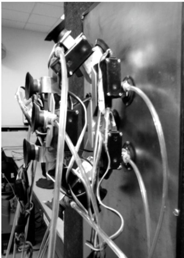
FIG. 6. "MARAK-I" DURING THE CHANGE OF STEPS OF WHEELING LOCOMOTION ON THE STEEL TEST BED
