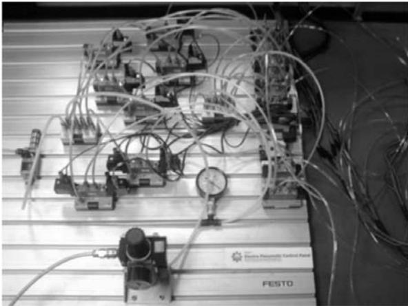
FIG. 5. "MARAK-I" PNEUMATIC ACTUATION MECHANISM
