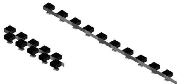
FIG. 2. MINIMUM POSSIBLE LENGTH FOR ZIG-ZAG AND LINEAR CONFIGURATIONS (TO ACHIEVE ROTATIONAL ASSUMPTIONS IN RECTILINEAR GAIT)
