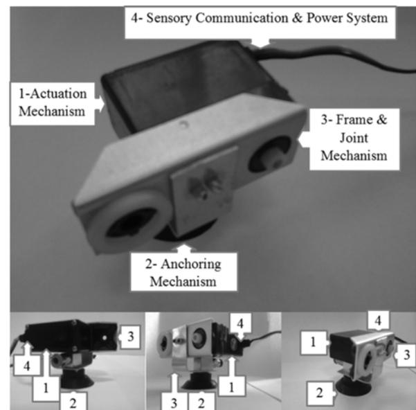
FIG. 1. MAJOR PARTS OF A MODULE OF "MARAK-I" ROBOT FROM DIFFERENT POINT OF VIEWS
