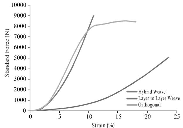
FIG. 2. TYPICAL FORCE - STRAIN CURVE OF 3D WOVEN STRUCTURES IN WEFT DIRECTION
