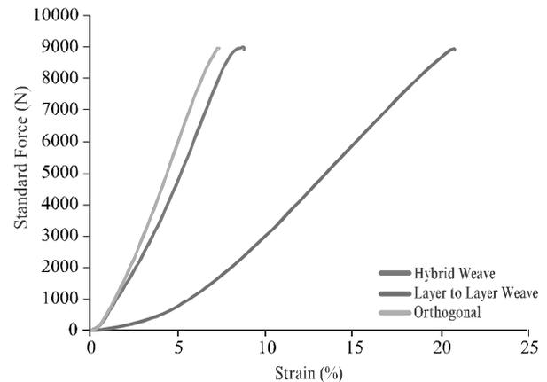
FIG. 1. TYPICAL FORCE-STRAIN CURVE OF 3D WOVEN STRUCTURES IN WARP DIRECTION
