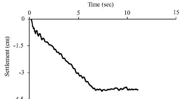
FIG. 13. SETTLEMENT OF LEFT (EXTERIOR) FOOTING VERSUS TIME
