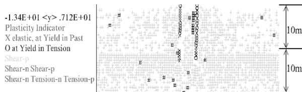
FIG. 11. PLASTICITY STATE OF COLUMNS FOR ONE ROW ADJACENT TO PAD
