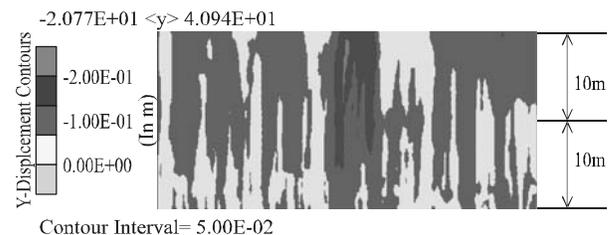
FIG. 10. VERTICAL DISPLACEMENT CONTOURS-ONE ROW ADJACENT TO EACH EDGE OF PAD
