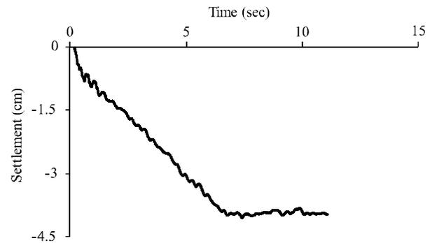
FIG. 14. SETTLEMENT OF CENTRAL (INTERIOR) FOOTING VERSUS TIME
