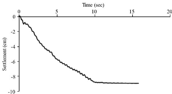
FIG. 5. SETTLEMENT OF FOOTING VS. TIME FOR ONE ADJACENT ROW
