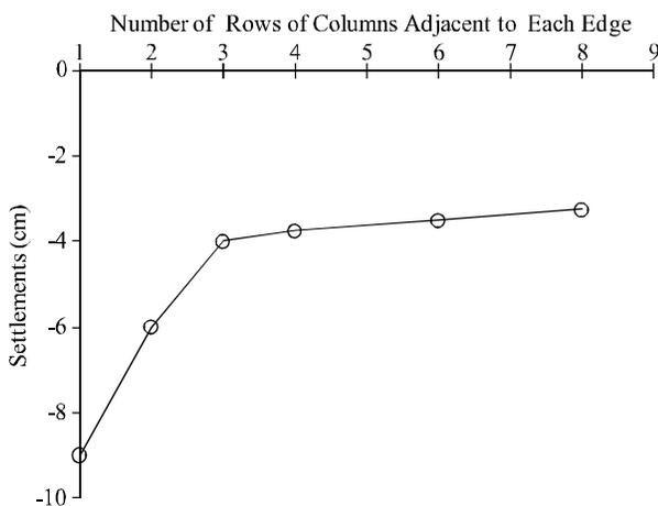
FIG. 9. SETTLEMENT VERSUS NUMBER OF ROWS OF COLUMNS ADJACENT TO THE FOOTING PAD
