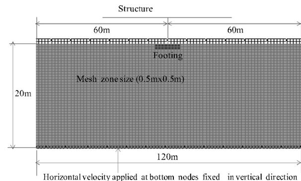
FIG. 3. FINITE DIFFERENCE MESH USED FOR FLAC 2D NUMERICAL ANALYSIS
