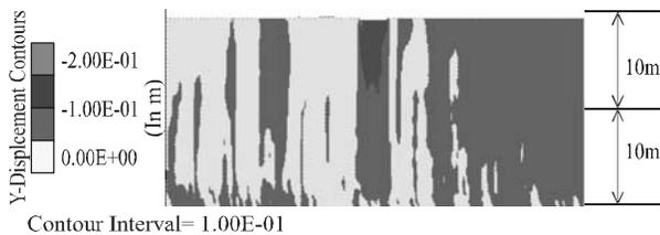
FIG. 8. VERTICAL DISPLACEMENT CONTOURS-THREE CONTINUOUS ROWS AT OFFSET OF 0.5m
