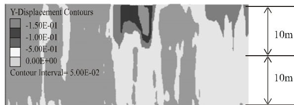
FIG. 9. VERTICAL DISPLACEMENT CONTOURS IN THE CASE FOR SHORT COLUMNS OF 4m LENGTH
