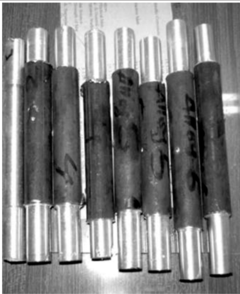
FIG. 8. STANDARD SPECIMENS PREPARED FOR TENSILE TEST
