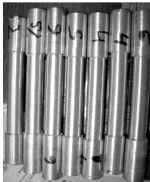
FIG. 8. STANDARD SPECIMENS PREPARED FOR TENSILE TEST
