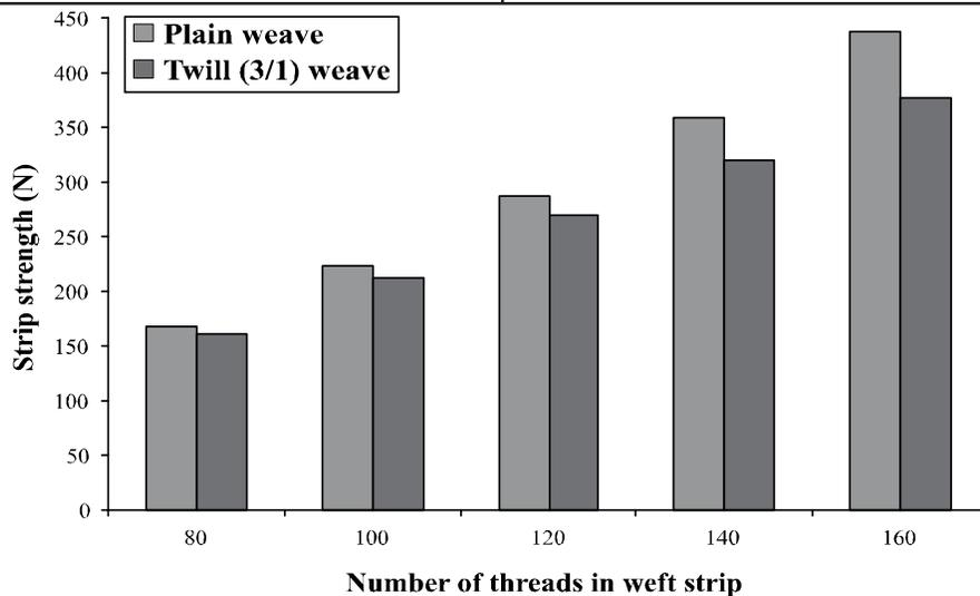
FIG. 2. COMPARISON OF WEFT WISE TENSILE STRENGTH FOR PC BLENDED FABRICS
