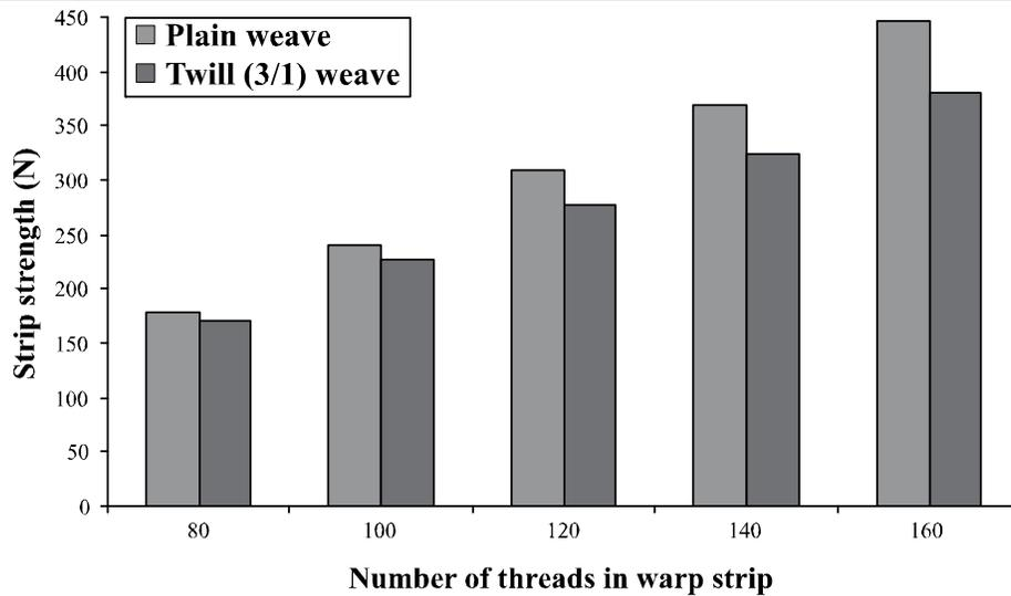
FIG. 1. COMPARISON OF WARP WISE TENSILE STRENGTH FOR PC BLENDED FABRICS
