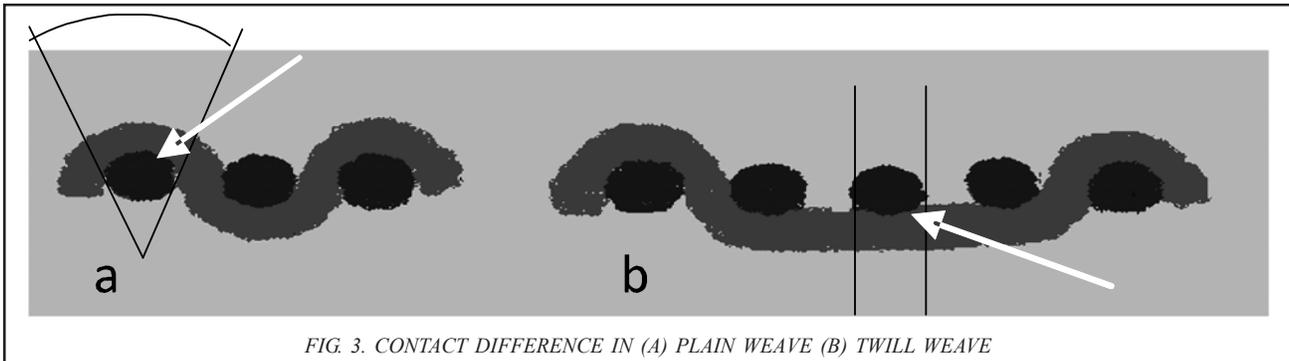
FIG. 3. CONTACT DIFFERENCE IN (A) PLAIN WEAVE (B) TWILL WEAVE
