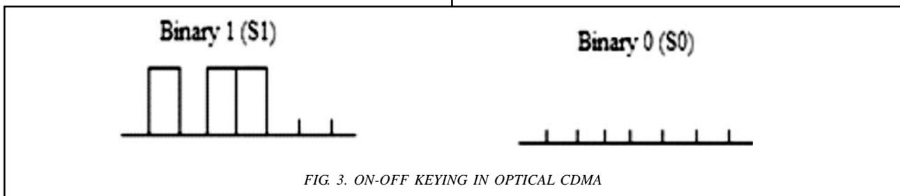
FIG. 3. ON-OFF KEYING IN OPTICAL CDMA
