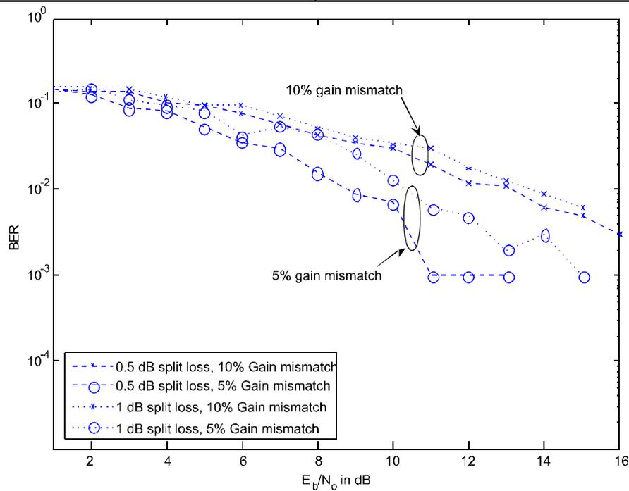
FIG. 7. BER VERSUS  $E_b/N_0$  FOR PDC-BASED OCDMA SYSTEM WITH BOTH APD GAIN MISMATCH AND SPLIT LOSS
