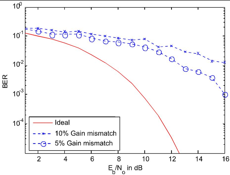
FIG. 5. BER VERSUS  $E_b/N_0$  FOR PDC-BASED OCDMA SYSTEM WITH GAIN MISMATCH ONLY.
