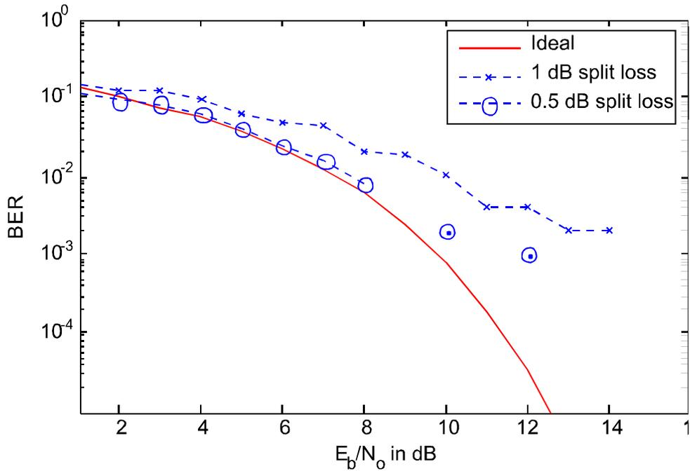
FIG. 6. BER VERSUS  $E_b/N_0$  FOR PDC-BASED OCDMA SYSTEM WITH SPLIT LOSS ONLY.
