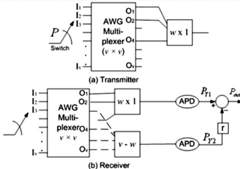
FIG. 1. SAC-OCDMA SYSTEM BASED ON PERFECT DIFFERENCE CODES [5]
