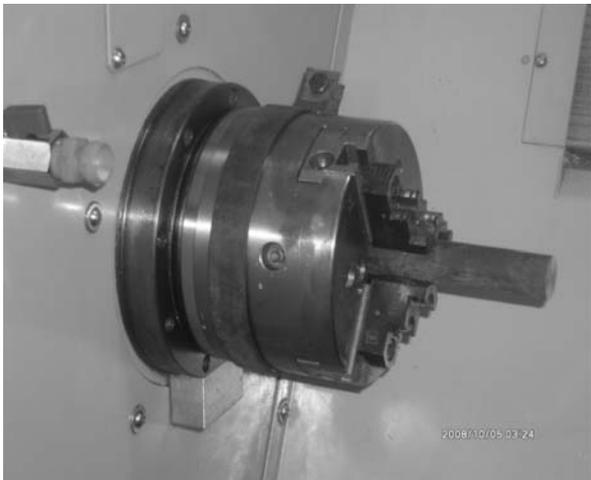
FIG. 1. UNBALANCED MASS ATTACHED TO MILD STEEL RING FASTENED ON THE CHUCK FOR GENERATING INDUCED LEVEL OF VIBRATION
