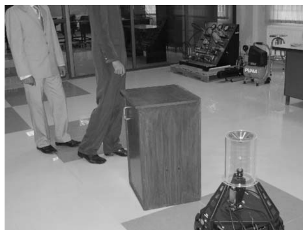
FIG. 6. EXAMPLE OF MOBILE ROBOT AVOIDING TWO DYNAMIC OBJECTS (PEOPLE) HIDDEN BY A STATIONARY OBJECT
