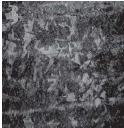
(c) MEDIUM BAINITE IN A SAMPLE AUSTEMPERED AT 350°C
