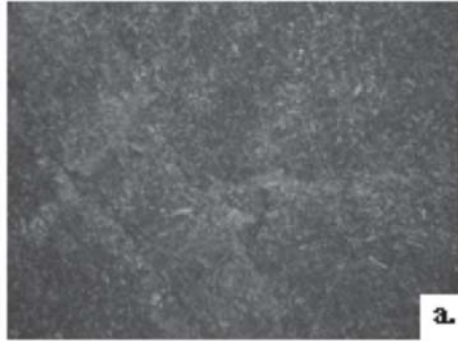
FIG. 1. MICROGRAPHS RECORDED AFTER TEMPERING AT (a) 480°C AND (b) 600°C X400
