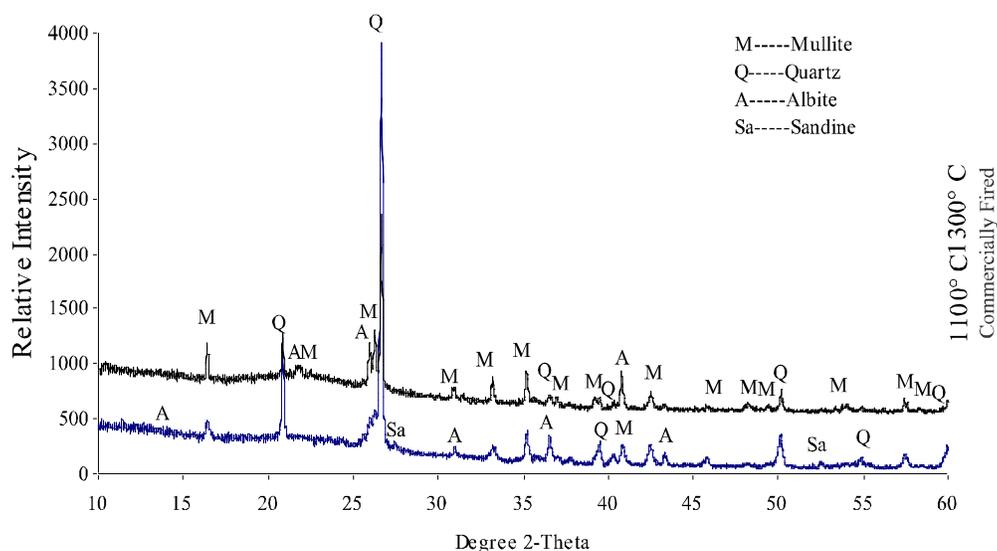
FIG. 2. XRD PATTERN OF SANITARY-WARE SAMPLES FIRED AT 1100 AND 1300°C
