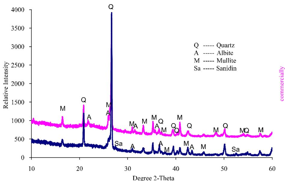
FIG. 1. COMPARISON OF XRD PATTERNS OF SANITARY-WARE SAMPLES FIRED COMMERCIALY AND AT 1100°C
