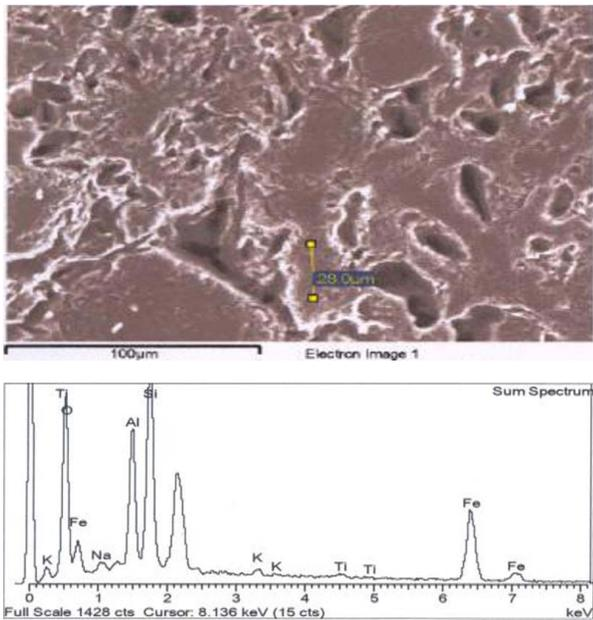
FIG. 5. SHOWS PRIMARY MULLITE OF SCALY APPEARANCE WITH REASONABLE AMOUNT OF IRON
