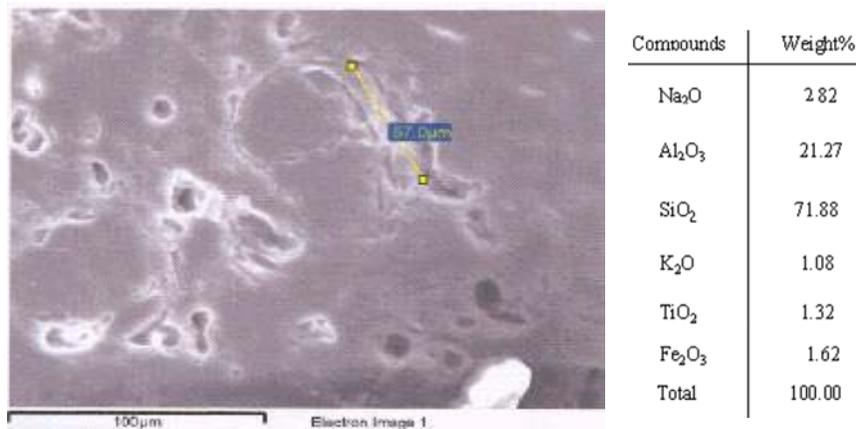
FIG. 8. SEI OF SAMPLE REHEATED AT 1200°C. THE EDS OF THE MARKED REGION REVEALS THE PRESENCE OF SILICA RICH MATRIX IN THE VICINITY OF α-QUARTZ GRAIN "Q" ALONG WITH OTHER IMPURITIES SUCH AS IRON, TITANIUM POTASSIUM. LABELS A, B AND C SHOW PRIMARY MULLITES
