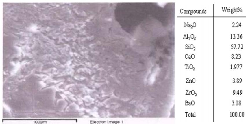
FIG. 9. GLAZE COMPOSITION AND MORPHOLOGY OF THE SAMPLE FIRED AT 1200°C
