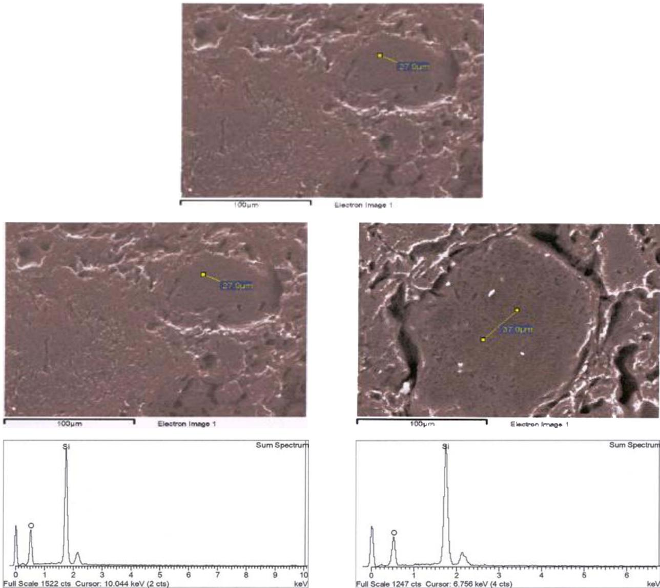
FIG. 4. AREAS SCANNED OVER 27.9 AND 37.0µm COMPRISES 100% SILICAAS CONFIRMED BY IN SET EDS SPECTRA
