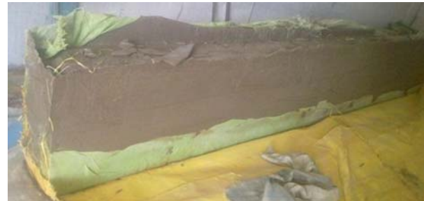
FIG. 3. A VIEW OF WALL MASONRY BLOCK IMMEDIATELY AFTER CASTING
