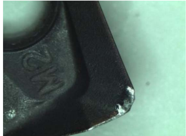
FIG. 15. TOOL WEAR IN DRY MACHINING
