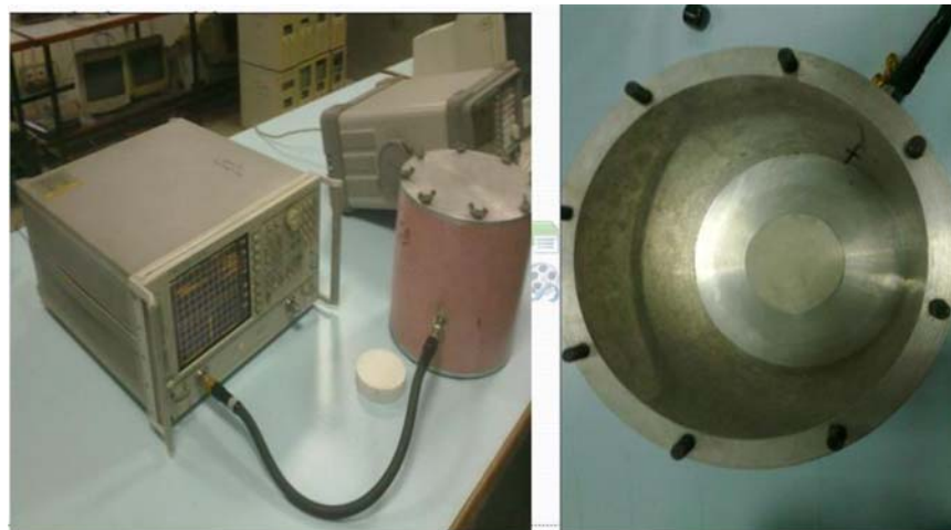
FIG. 9. NETWORK ANALYZER MEASUREMENT SETUP
