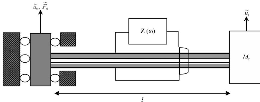
FIG. 2. DIRECTION-FIXED BASE/TIP FREE CANTILEVER BEAM WITH END MASS
