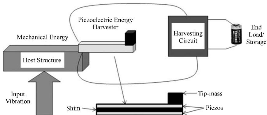
FIG. 1. BLOCK DIAGRAM OF A TYPICAL PVEH MECHANISM [1]
