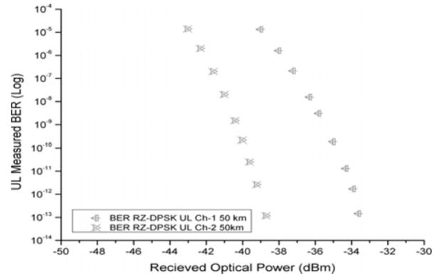
FIG. 8. BER GRAPH FOR RZ-DPSK UL CHANNELS (50KM)
