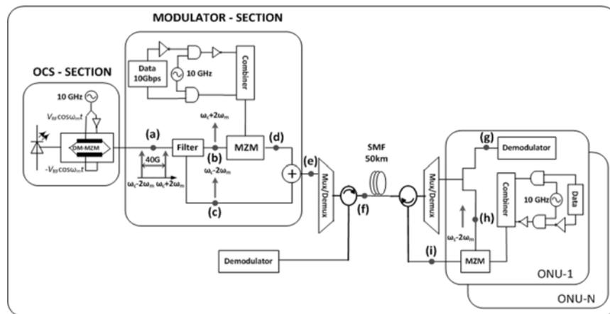
FIG. 3. SCHEMATIC DIAGRAM OF PROPOSED WDM-PON ARCHITECTURE
