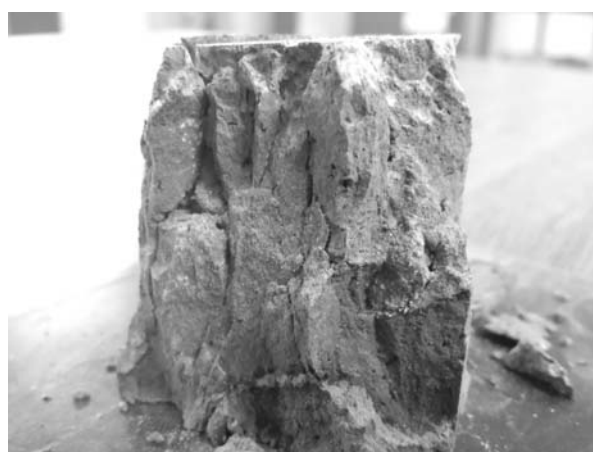
FIG. 7. CUBE CUT FROM BAKED CLAY BRICK OF BARA HAZARI AND TESTED IN UNIVERSAL TESTING MACHINE
