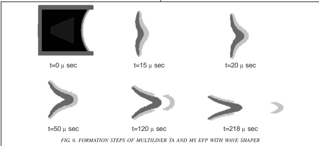
explosive to make planer shock wave that struck normal to the liner material then these two materials were separated after 130  $\mu$ sec. Hence, the waveshaper has prominent and faster tandem effect on the multiliner EFPs. The cylindrical and tapered casings have no effect on multiliner EFP.
