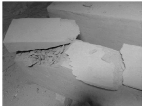
*FIG. 1. CRACKING OF CLAY BEAMS DURING FIRING IN THE LABORATORY KILN*
