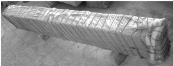
*FIG. 5 THE CLAY BEAM BEING WOUND BY JUTE ROPE AFTER COVERING WITH PLASTIC SHEET*
