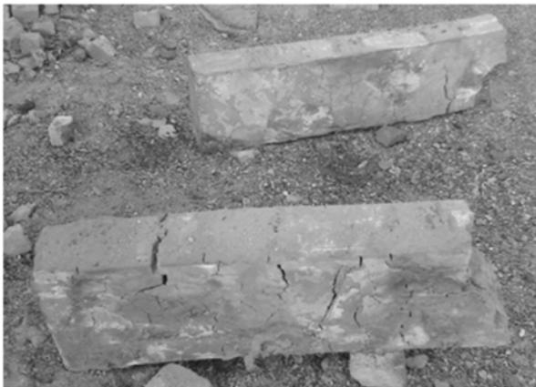
*FIG. 2. THE BEAMS BAKED IN THE COMMERCIAL KILN WITHOUT APPLYING ANY TREATMENT*
