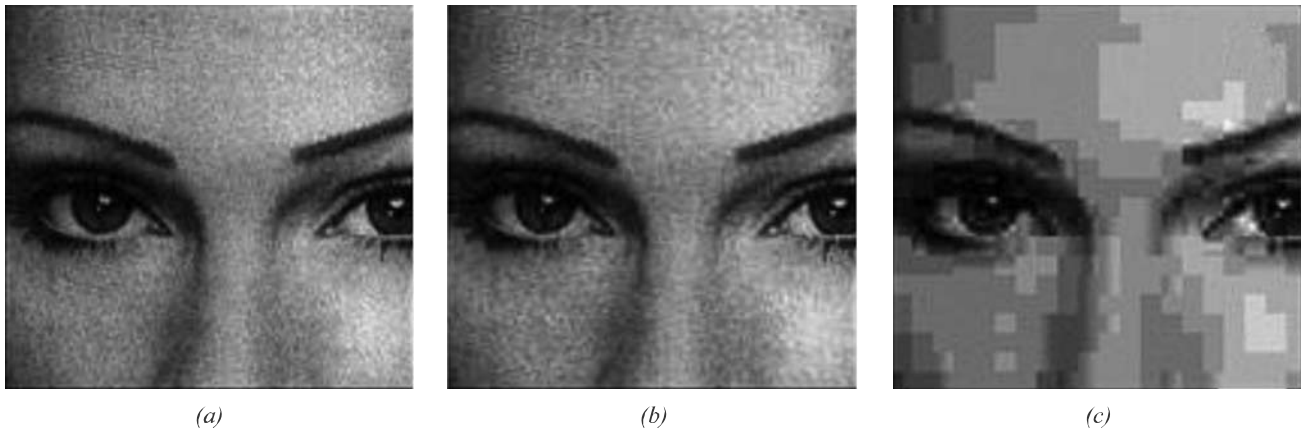
FIG 4.(a) THE ORIGINAL REF IMAGE [9], (b-c) SHOW IMAGES WITH THE COMPRESSION RATIO OF 10.0:1.0 AND 45.0:1.0 RESPECTIVELY.
