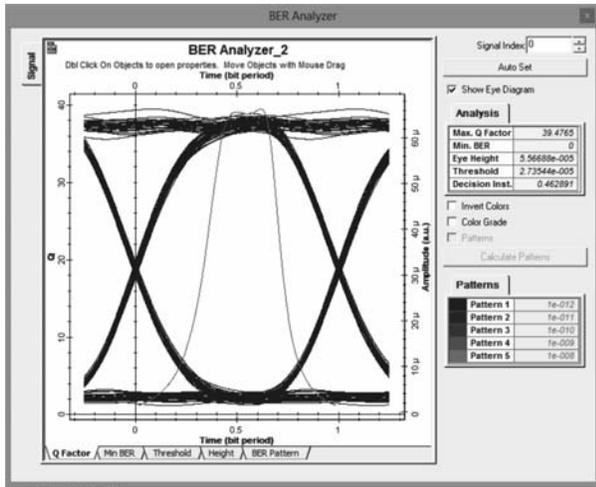
FIG. 13. MAX Q AND EYE PATTERN OF 1570 NM
