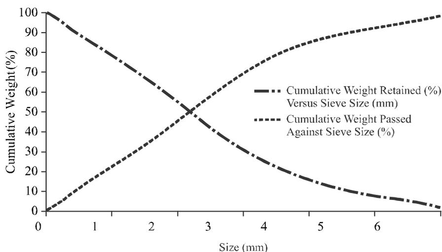
FIG. 1. SIEVE ANALYSIS OF CRUSHED PRODUCT
