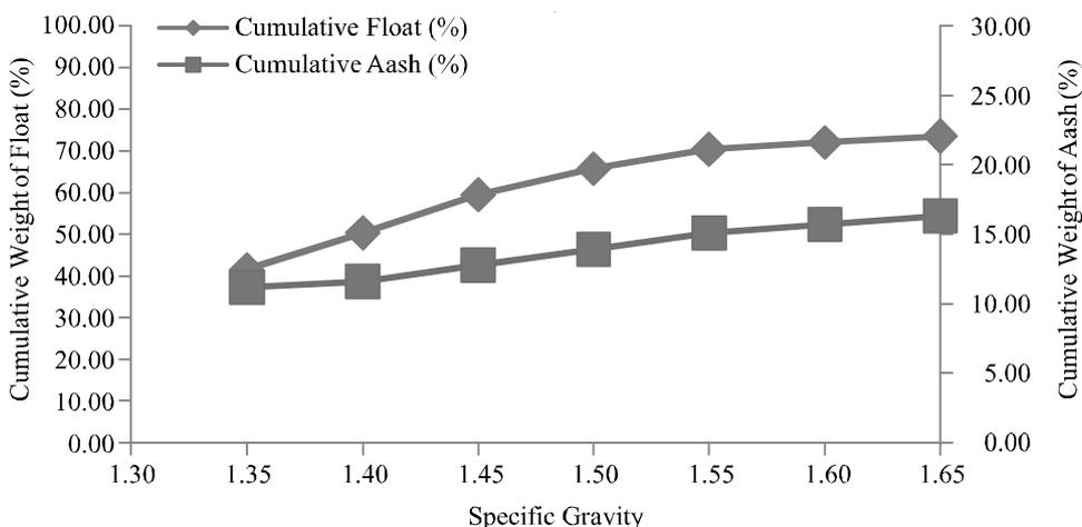
FIG. 5(a). WASHABILITY CURVES FOR SIZE FRACTION -3.35 + 1.4mm SHOWING CHANGE IN ASH CONTENT
