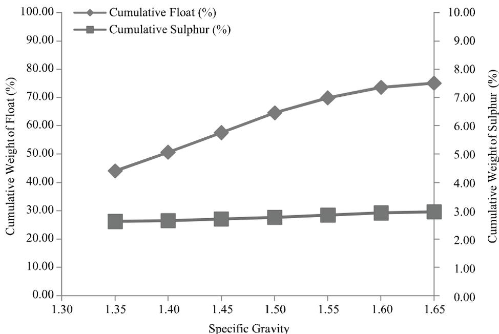
FIG. 3(b). WASHABILITY CURVES FOR SIZE FRACTION -0.71+0.5mm SHOWING CHANGE IN SULPHUR CONTENT
