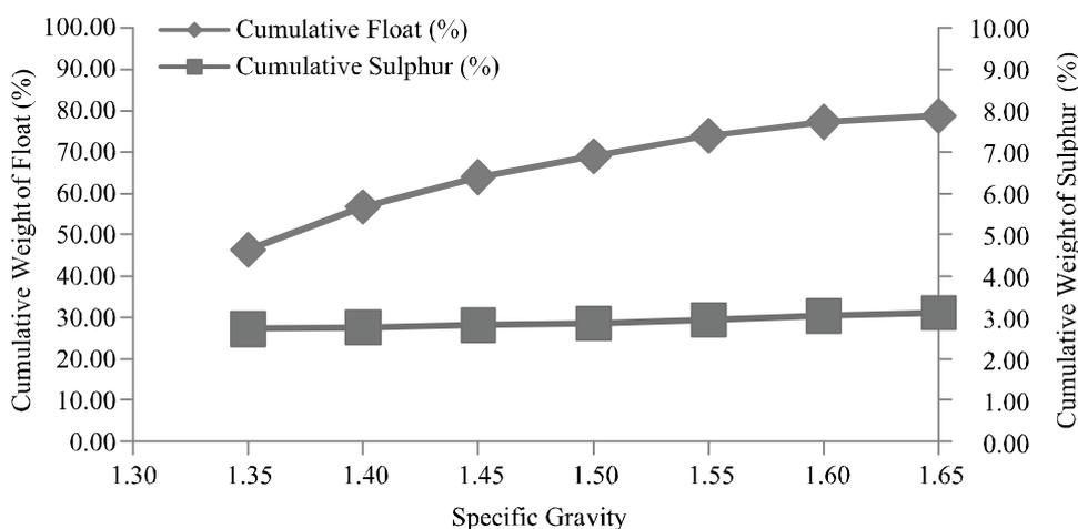
FIG. 4(b). WASHABILITY CURVES FOR SIZE FRACTION - 1.4+0.71mm SHOWING CHANGE IN SULPHUR CONTENT
