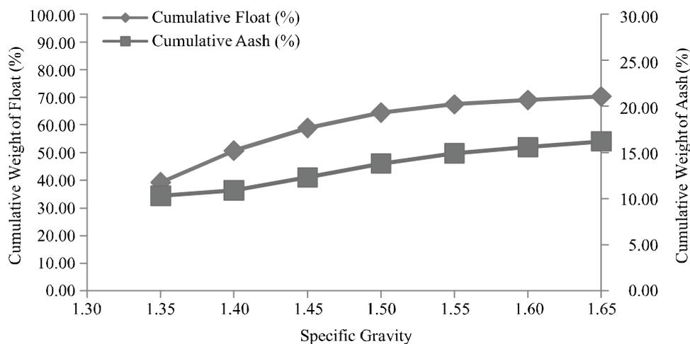
FIG. 6(a). WASHABILITY CURVES FOR SIZE FRACTION -5.6+3.35 mm SHOWING CHANGE IN ASH CONTENT
