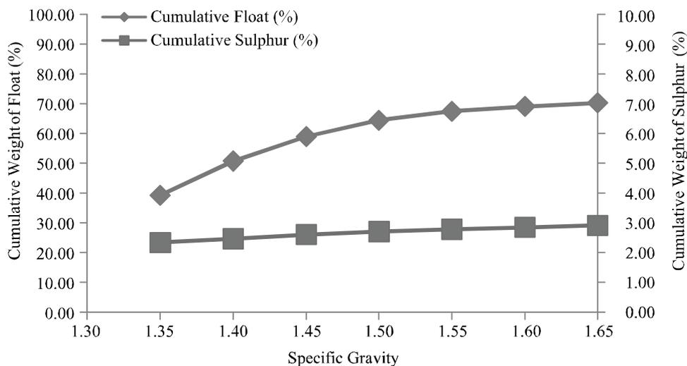
FIG. 6(b). WASHABILITY CURVES FOR SIZE FRACTION -5.6+3.35mm SHOWING CHANGE IN SULPHUR CONTENT
