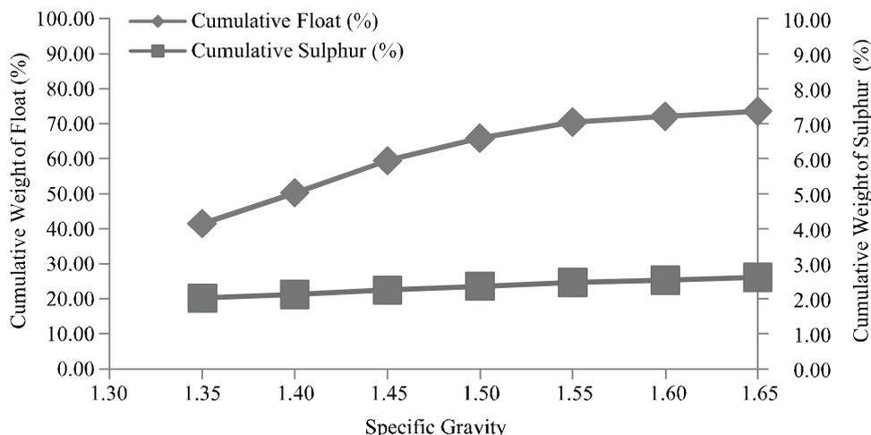
FIG. 5(b). WASHABILITY CURVES FOR SIZE FRACTION -3.35 + 1.4mm SHOWING CHANGE IN SULPHUR CONTENT
