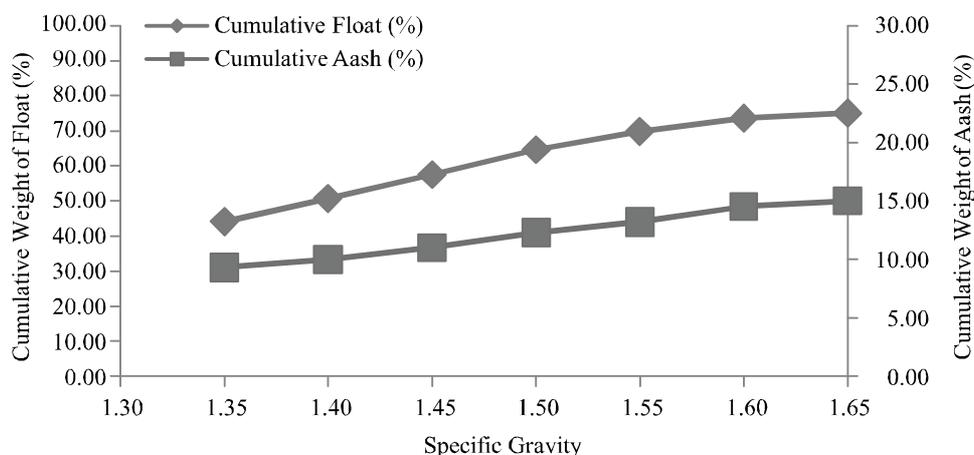
FIG. 3(a). WASHABILITY CURVES FOR SIZE FRACTION -0.71+0.5mm SHOWING CHANGE IN ASH CONTENT
