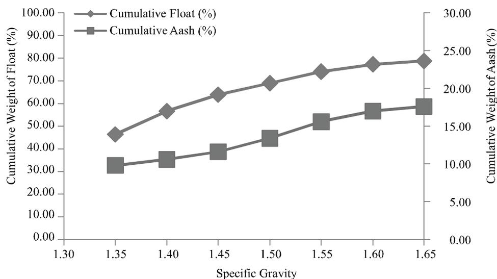
FIG. 4(a). WASHABILITY CURVES FOR SIZE FRACTION - 1.4+0.71mm SHOWING CHANGE IN ASH CONTENT
