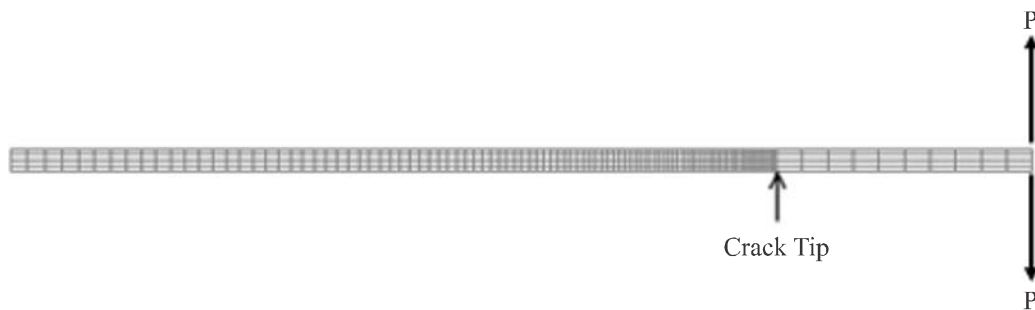
FIG. 5. MESH DIAGRAM OF DCB SPECIMEN
