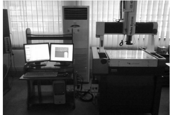
FIG. 5. COORDINATE MEASURING MACHINE USED FOR EDGE QUALITY MEASUREMENTS
