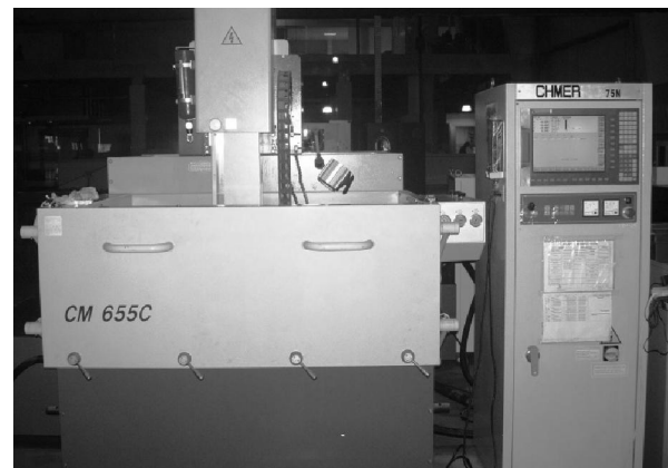
FIG. 2. ELECTRICAL DISCHARGE DIE SINKING MACHINE USED FOR EXPERIMENTATION
