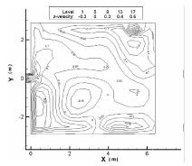
FIG. 11(b). Z-VELOCITY CONTOURS LES T=5600SEC
