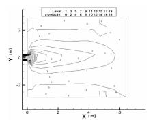
FIG. 4(a). X-VELOCITY CONTOURS LES T=5600 SEC
