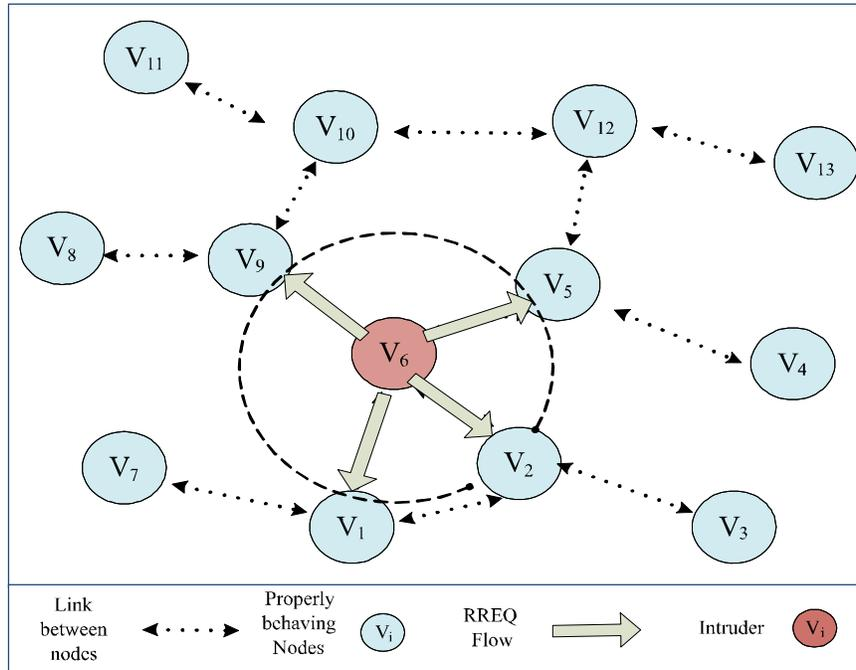
FIG. 2. SNAPSHOT OF NETWORK AFTER INTRUDER GENERATE MRREQ [5]
