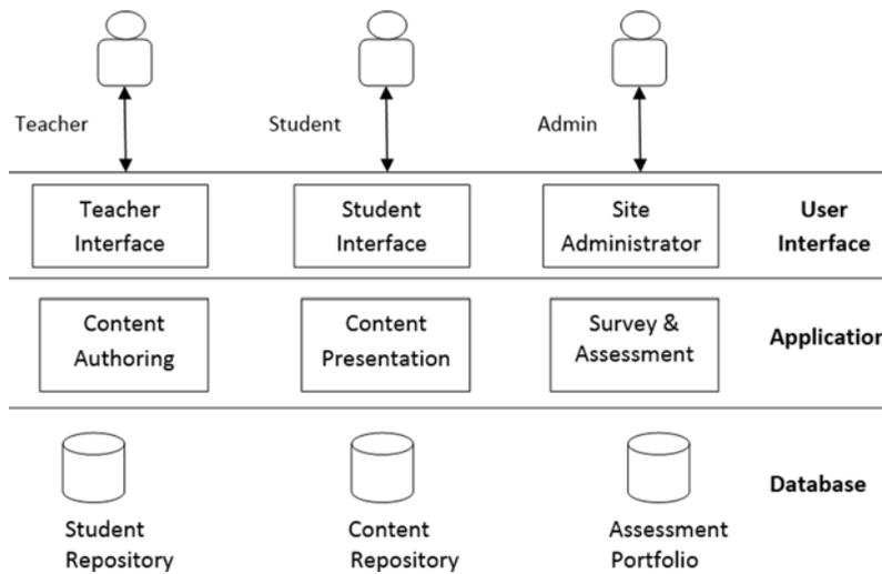
FIG. 5. THREE TIER CLIENT/SERVER ARCHITECTURE OF ADAPTIVE E-LEARNING MODEL
